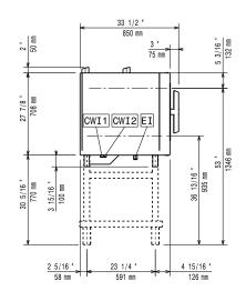
CWI1 = Cold Water inlet 1 (cleaning) CWI2 = Cold Water Inlet 2 (steam
